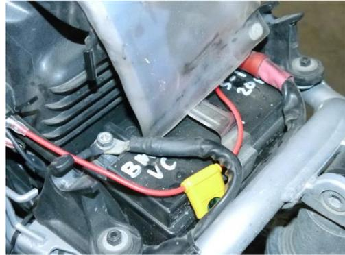
**Step 2:** Route the battery terminal lead harness to the front of your bike so the harness with the relay plugs in behind your stock headlight.
