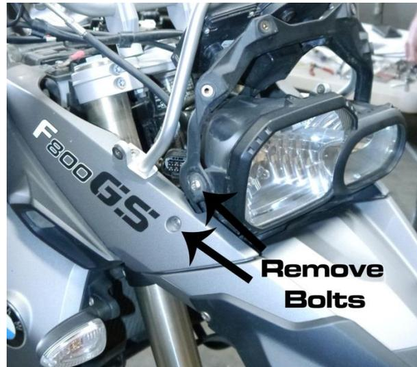
**Step 2:** Once those bolts have been removed, locate the mounting brackets, spacer and reduced flange head bolts which have been included in this kit. Once you have located all of those parts, refer to the drawing below for the installation order.
